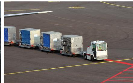
The Tennessee Valley Authority (TVA) partnered with four airports in the Valley and FedEx in 2016 to replace a portion of their diesel-powered ground support equipment (GSE) with no-emission, all-electric gear. Airport GSE includes tugs for airplane pushback and hook-up, carts for moving people and materials, air conditioning tugs that provide power to the aircraft, belt and container loaders, and other equipment. Electric GSE has zero exhaust emissions and can greatly reduce NOx emissions.
