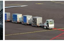
The Tennesee Valley Authority (TVA) partnered with four airports in the Valley and FedEx in 2016 to replace a portion of their diesel-powered ground support equipment (GSE) with no-emission, all-electric gear. Airport GSE includes tugs for airplane pushback and hook-up, carts for moving people and materials, air conditioning tugs that provide power to the aircraft, belt and container loaders, and other equipment. Electric GSE has zero exhaust emissions and can greatly reduce NOx emissions.
